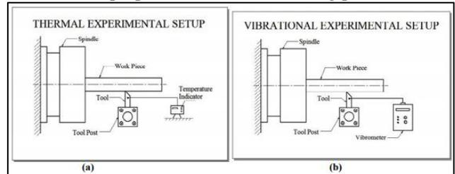
Fig. 8: Schematic Showing Experimental Setup (a) For Thermal Analysis and (b) For Vibration Analysis
