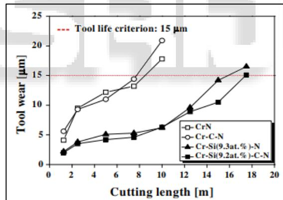
Fig. 9: Variation of Flank Wear of CrN, Cr-C-N, Cr-Si-N, and Cr-Si-C-N Coated Micro End-Mill as Function of Cutting Length
