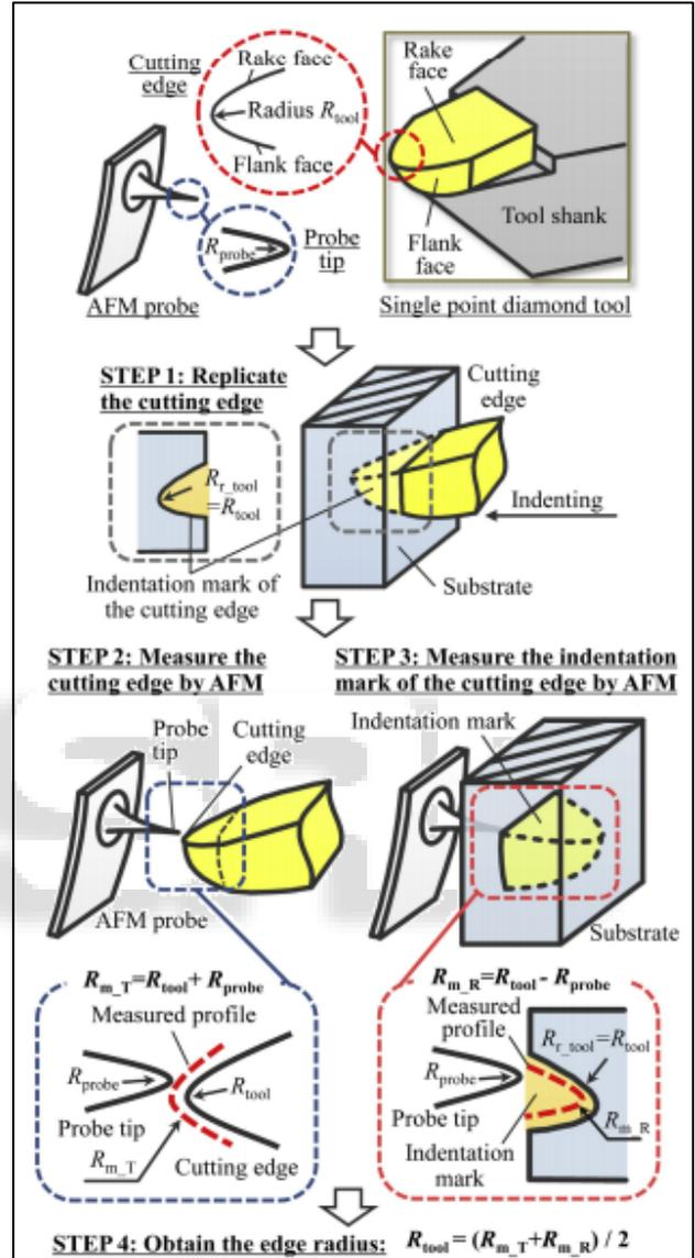
Fig. 5: Schematic of the edge Reversal Method Proposed for Precision Measurement of the Cutting Edge Radius of a Single Point Diamond Tool
