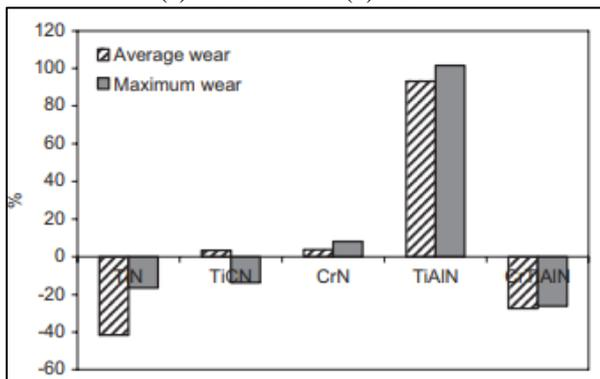
Fig. 7: Comparison of Wear between Coated and Uncoated Tools
