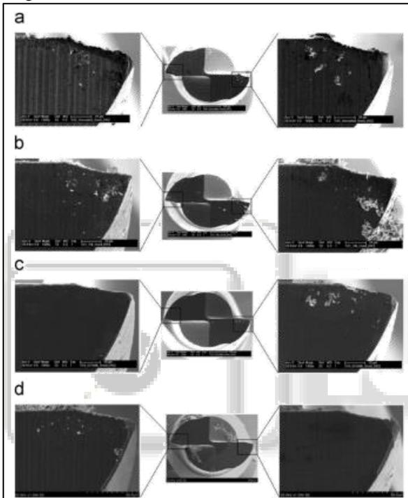
Fig. 6: Wear on Tool after Machining (a) Uncoated, (b) TiN, (c) CrTiAlN and (d) TiAlN
