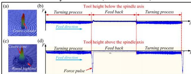
Fig. 4: Centre Cylinder and Cone Appearances and Corresponding Cutting Force Forms
