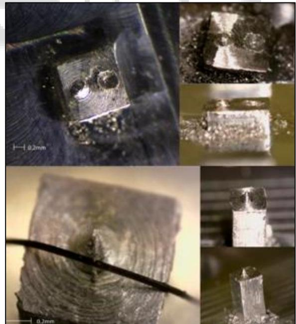
Fig. 14: Micro Geometries Obtained with the 3PRS+XY+C Micro Machine Tool. Top Image Shows a Concave and Convex Dome, the Bottom Image shows a Micro Cone Compared to a Human Hair
