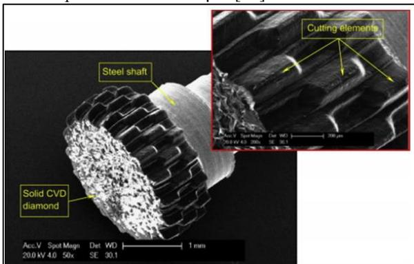
Fig. 15: Unused Laser Ablated Solid Diamond Micro-Grinding Tool [11]
