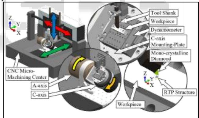
Fig. 1: Experimental Setup: Five-Axis Micromachining Center, Tool, Dynamometer, & Workpiece
