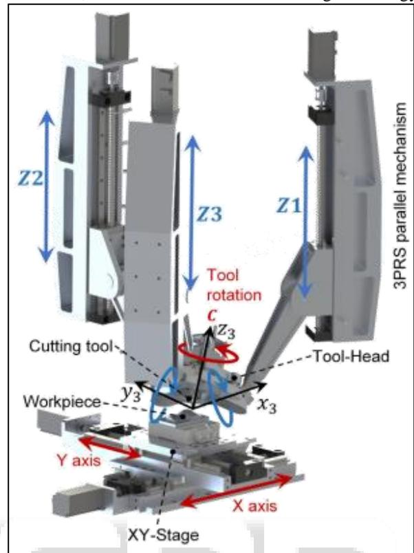
Fig. 13: Geometrical Model of the 3PRS+XY+C Hybrid Machine Tool
