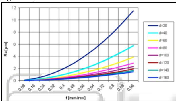
Fig. 11: Graphical form of  $Rz_1$  value for Oblique Turning ( $\lambda_s=60^\circ$ ) with Single-Edge, Depending on the Feed and the Diameter of the Work Surface
