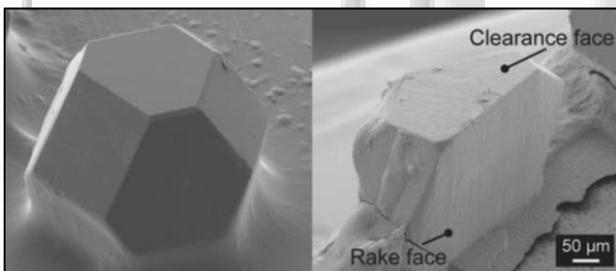
Fig. 16: Diamond Grain Shaped by Laser for EGT Applications
