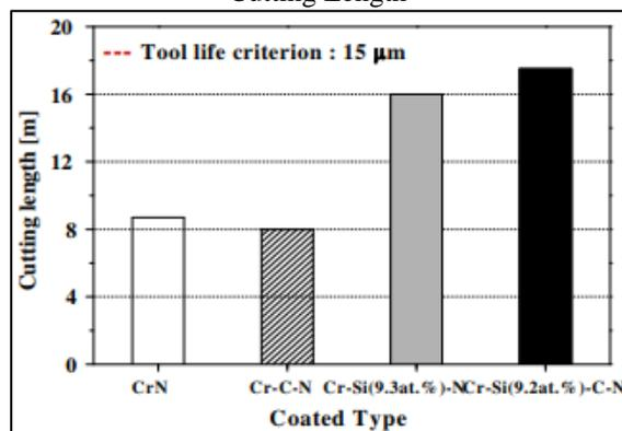
Fig. 10: Comparison of Tool Life According to CrN, Cr-C-N, Cr-Si-N, and Cr-Si-C-N Coated Micro End-Mill
