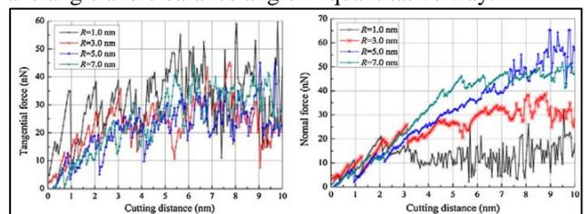
Fig. 18: Variation of the Cutting Forces with Cutting Distance for different Tool Edge Radius
