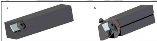
Fig. 12: MCAD 3D Models of Tools for Oblique Cutting with Straight Cutting edge: a) the Tool with a Permanent Geometry of edge, b) a Tools with Moveable cutting Edge with an Option to Change  $\lambda R_s R$  angle
