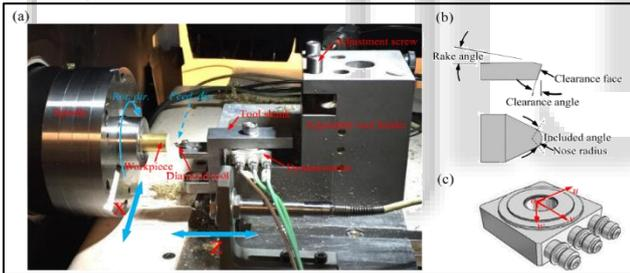
Fig. 3: (A) Experimental Setup, (B) Geometric Parameters of Diamond Tools and (C) Force Component Directions of the Dynamometer (Kistler 9252A)
