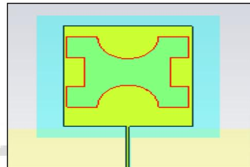
(A) Design of Front View of Multilayer Microstrip Monopole Fractal Patch Antenna
