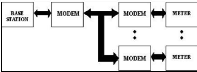
Fig. 2: AMR Communication Setup
