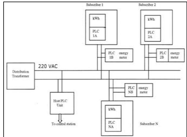
Fig. 3: Schematic Illustration of Detection System of Illegal Electricity Usage
