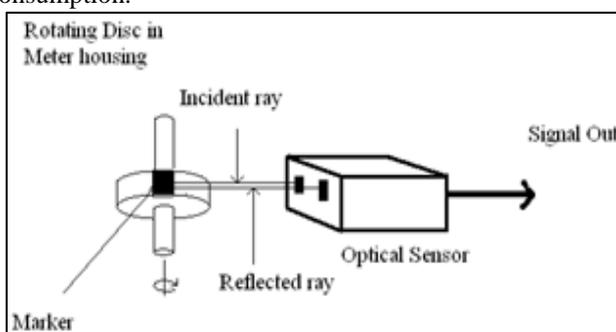
Fig. 1: Electromechanical Movement to Digital Signal Conversion
