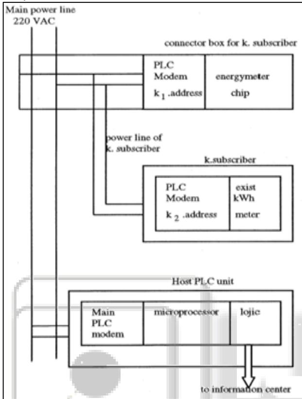
Fig. 4: Illegal Detector System of One Sub-Subscriber
