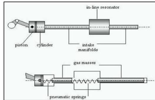
Fig. 5: Equations of double Helmholtz resonator and double engine with in-line resonator representation
