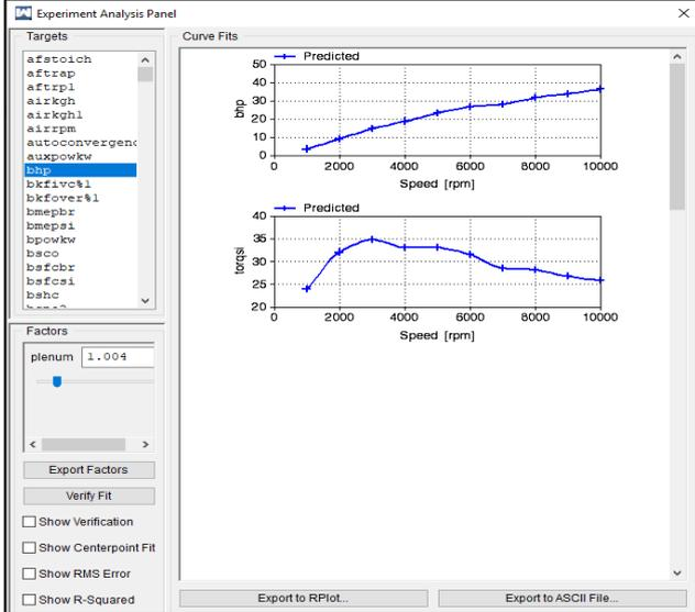
Fig. 7: Bhp and Torque curve for 1000cc plenum
