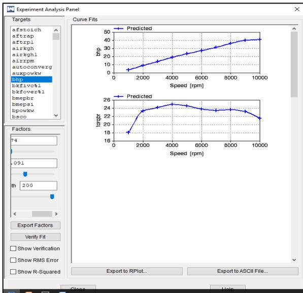
Fig. 10: Bhp and torque curve of final configuration
