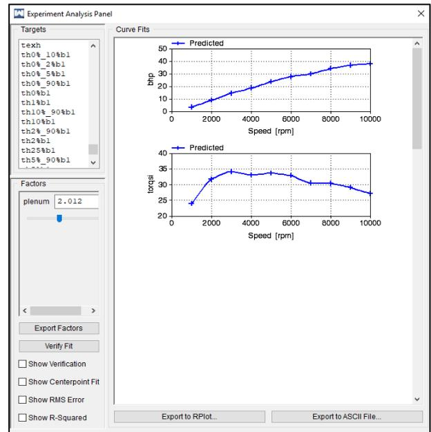
Fig. 8: Bhp and Torque curve for 1500cc
