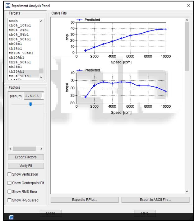
Fig. 9: Bhp and Torque curve for 2500cc plenum
