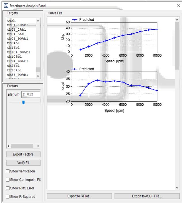
Fig. 8: Bhp and Torque curve for 1500cc plenum
