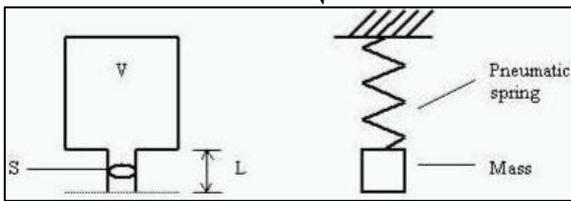
Fig. 4: Helmholtz Resonator Analogy
