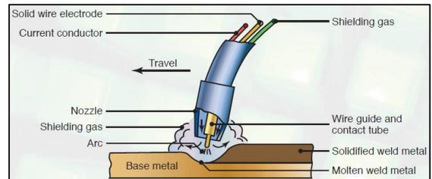
Fig. 1: Schematic Diagram of GMAW Welding System
