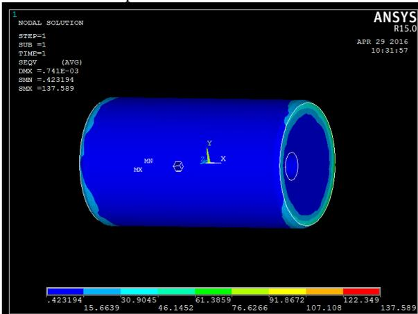
Fig. 6: Von Mises Stress at 1.5 mm Depth
