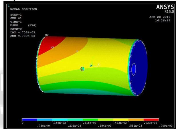
Fig. 5: Displacement Result of Crankpin
