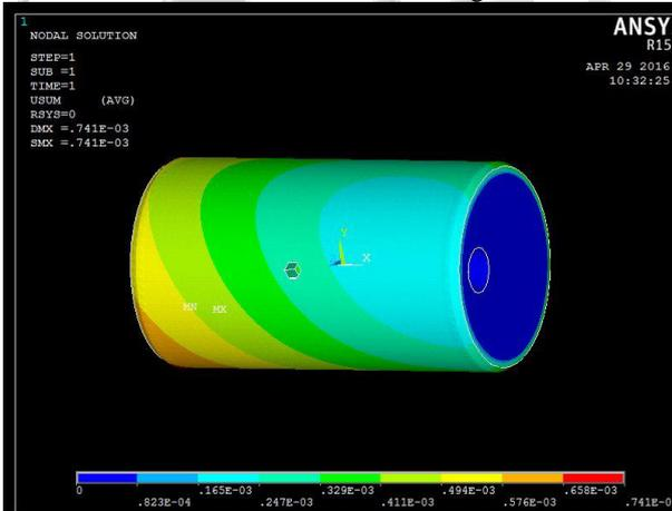
Fig. 7: Displacement Result of the Crankpin
