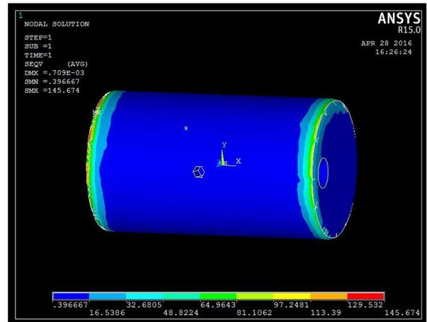
Fig. 4: Von Mises Stress of ADI for Crankpin
