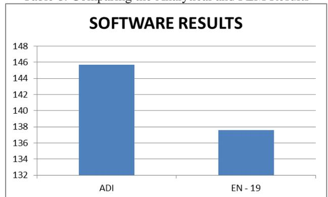
Fig. 8: Von mises stress result in N/mm<sup>2</sup>
