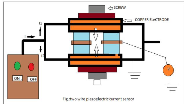
Fig. 2: Two wire Piezoelectric current sensor
