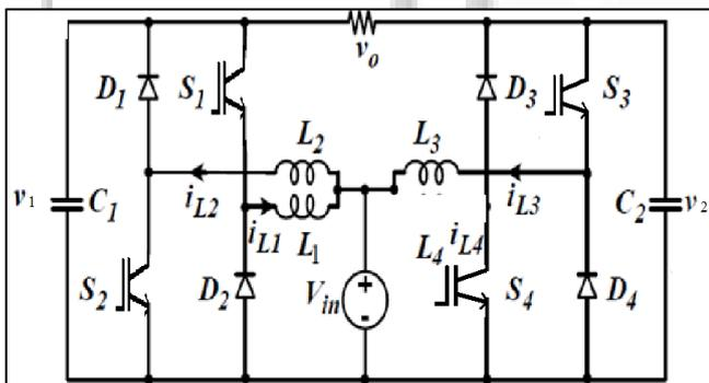
Fig. 4: Proposed Single –Phase Buck-Boost Inverter
