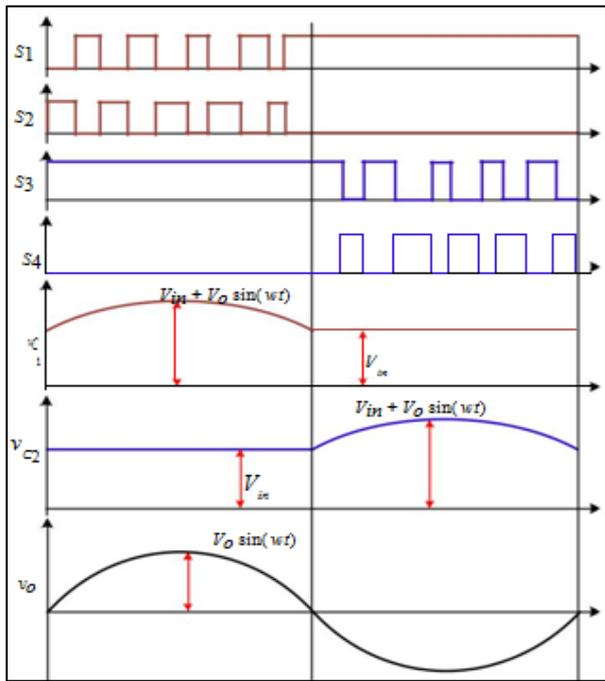
Fig. 5: Half-Cycle PWM Switching Scheme
