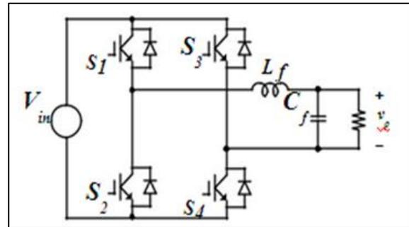
Fig. 1: Traditional Voltage Source Inverter
