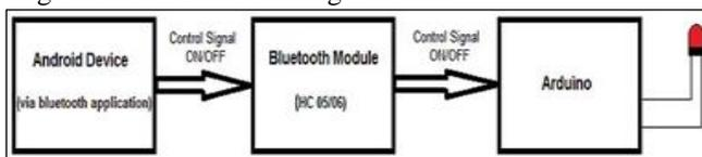
Fig. 3: Module block diagram
