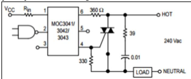
Fig. 4: Switching of TRIAC by Optocoupler
