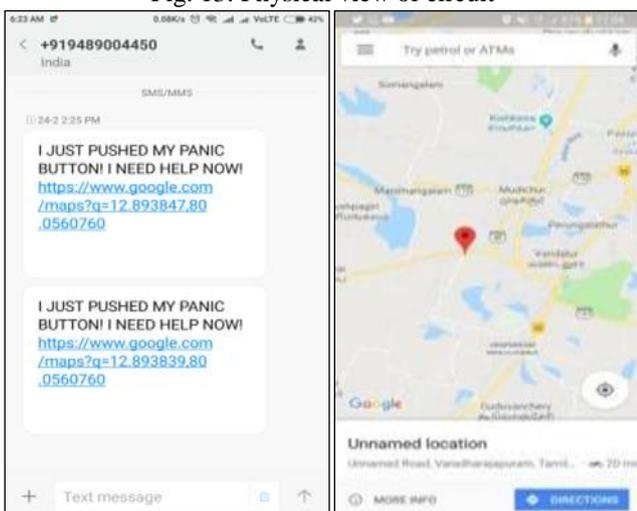
Fig. 14: SOS Message and Location of the device
