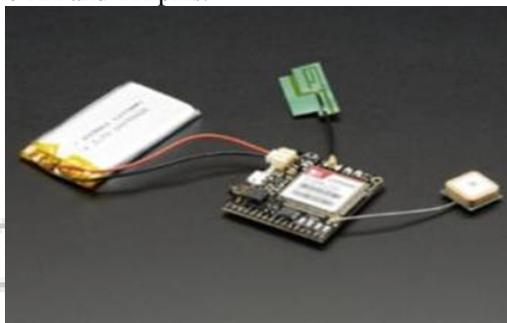
Fig. 4: Connection of antennas and battery with SIM808
