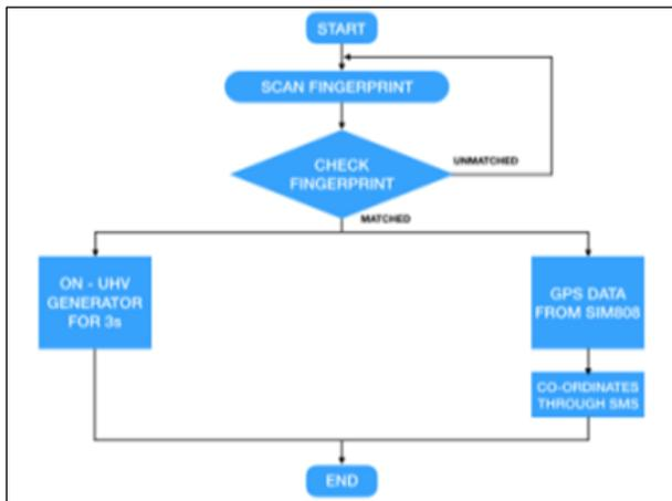
Fig. 12: Flowchart for software program approach
