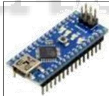
Fig. 2: Arduino nano board
