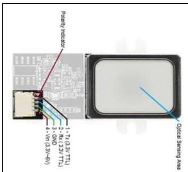
Fig. 5: Fingerprint Scanner
