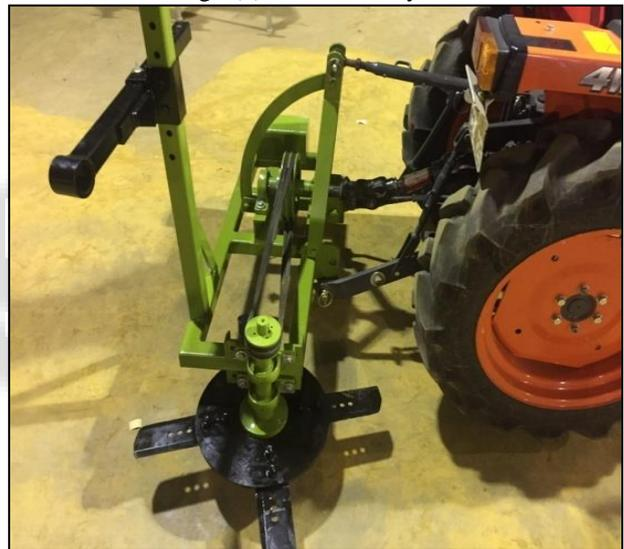
Fig. 2(c): Low Cost Sugarcane Cutting Machine
