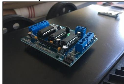
Fig. 4: Motor Shield
