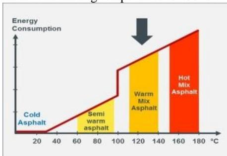
Fig. 1: Graphical Presentation of Temperature Range of Bituminous Mix
