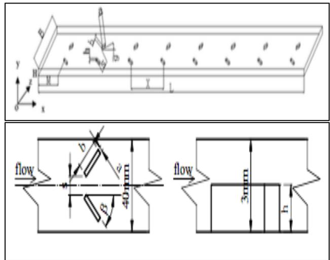
Fig. 7: (a) Schematic of narrow rectangular channel with 8 pairs LVGs, (b) Top view and side view of LVGs[40]
