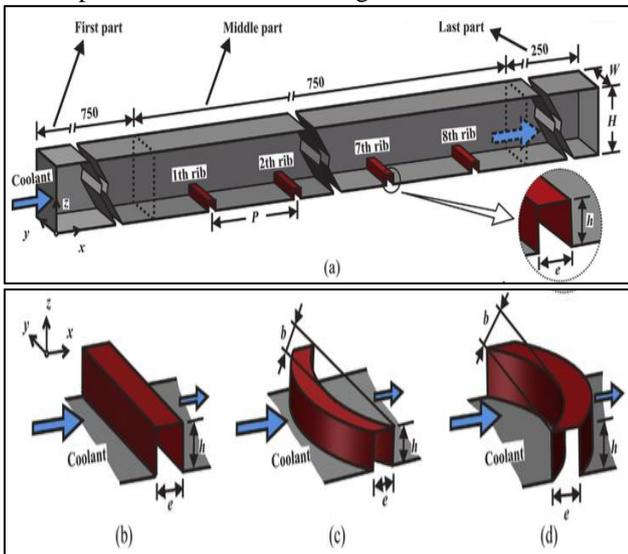
Fig. 2: Computational domain: (a) an overview of the cooling channel; (b-d) schematic illustration of the cooling channel with (b) straight rib (Case A), (c) crescent rib concave to the stream-wise direction (Case B) and (d) crescent rib convex to the stream-wise direction (Case C), respectively. [24]
