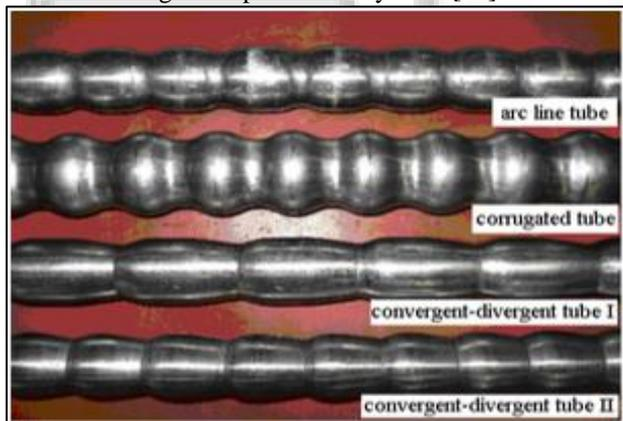
Fig. 6: Picture of enhanced tubes. [39]
