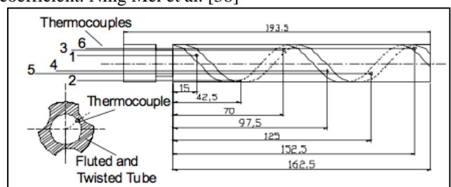
Fig. 4: Sketch of thermocouples embedded scheme. [38]
