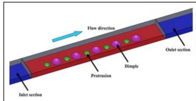
Fig. 1: A schematic diagram of the investigated rectangular channel [17]
