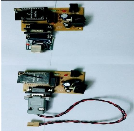
Fig. 5: Zigbee Transmitter and Receiver
