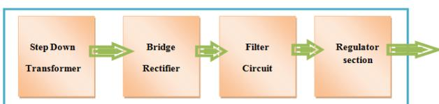
Fig. 1: Block Diagram of Power supply
