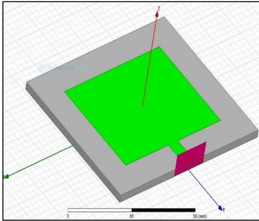
Fig. 2(a): Microstrip Patch Antenna with Single Layer
