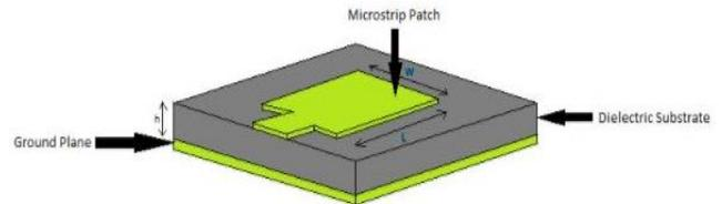
Fig. 1: Structure of Microstrip Patchb Antenna
