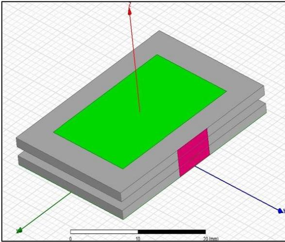
Fig. 3(a): Double Layer Microstrip Stack Antenna.
