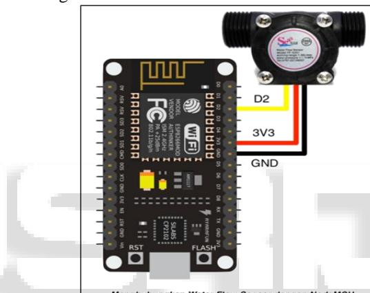
The data of discharge of the water is used to map the total discharge graph on the Android phone and also acts as feedback to the module controlling the motor rotation. From the feedback of the Flow Sensor the valve position can be determined corresponding to the specified amount of discharge.
