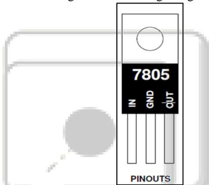
Fig. 6: Pin out Diagram of 7805 IC
