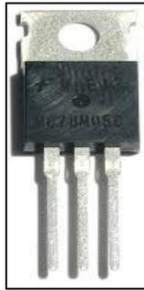
Fig. 5: 7805 Voltage Regulator IC
