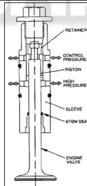
Fig. 7: Engine valve
