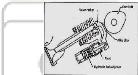
Fig. 3: Conventional Valve Train Mechanism
