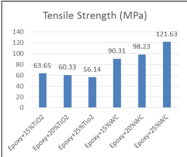
Fig. 2: Effect of fillers on tensile strength
