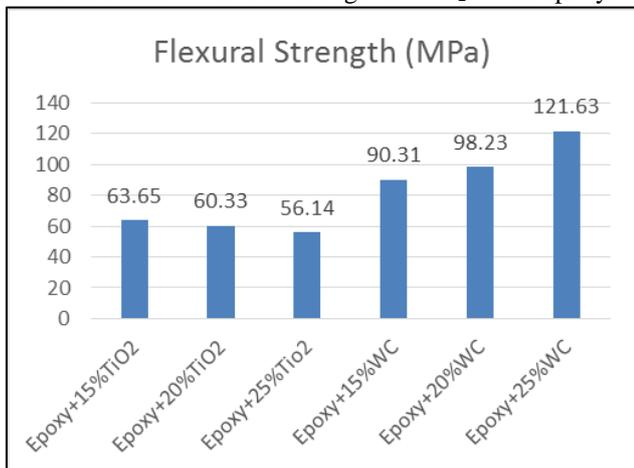
Fig. 3: Effect of fillers on flexural strength
