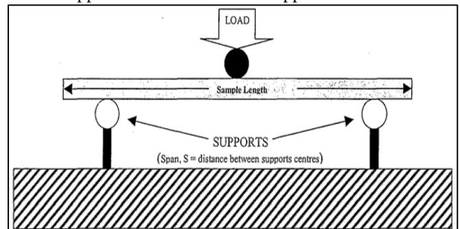
Fig. 1: 3 Point bending test
