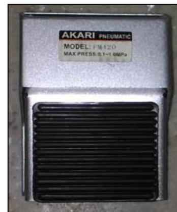
Fig. 3: Foot pedal mechanism
