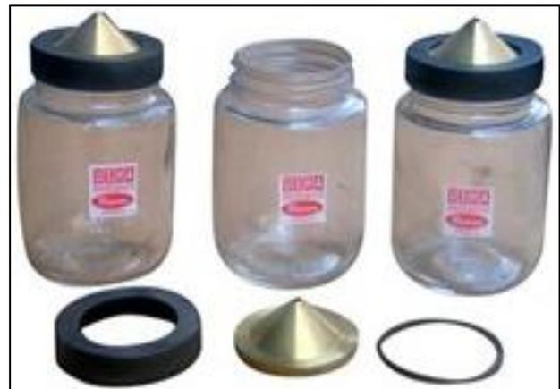
Fig. 4: Pycnometer Bottles
