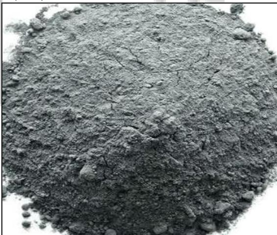
Fig. 3: Fly Ash Sample
