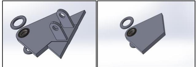
Fig. 9: Lower and Upper attachment parts respectively of version 04
