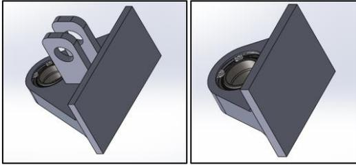
Fig. 7: Lower and Upper attachment parts respectively of version 03
