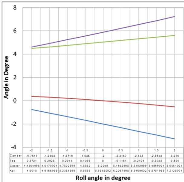
Fig. 3: Front Suspension Roll Analysis
