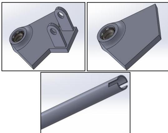
Fig. 8: Lower and Upper attachment parts and slotted tube respectively of version 03
