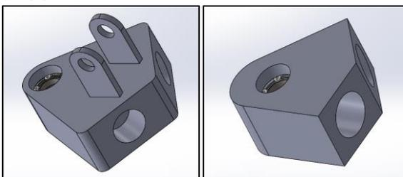
Fig. 5: Lower and Upper attachment parts respectively of version 01
