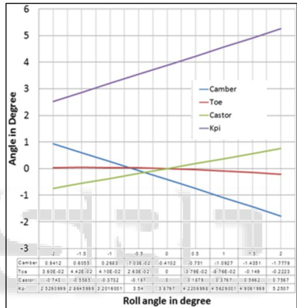
Fig. 1: Rear Suspension Roll Analysis
