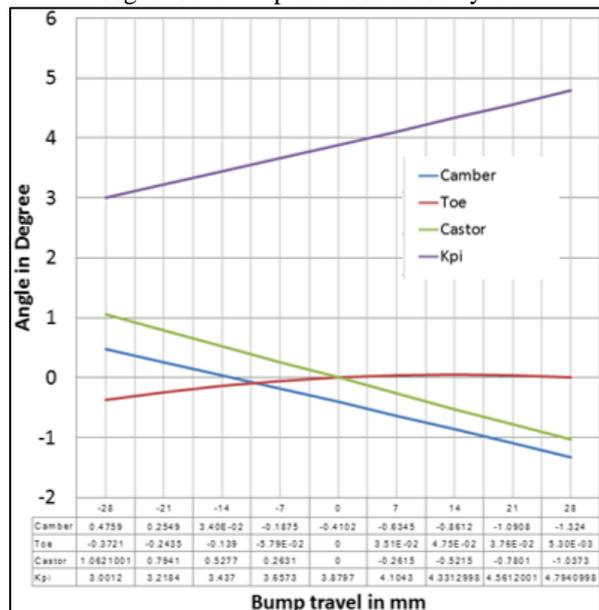
Fig. 2: Rear Suspension Bump Analysis
