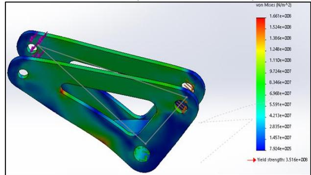
Fig. 12: Static FEA Analysis of Rocker Arm
