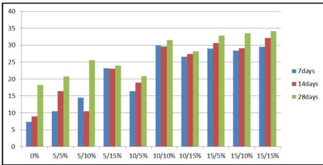
Fig. 3: Flexural strength at 7, 14 and 28 days
