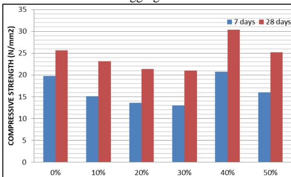
Fig. 4: Compressive Strength of M25 Concrete For Different Percentages Of Recycled Coarse Aggregate
