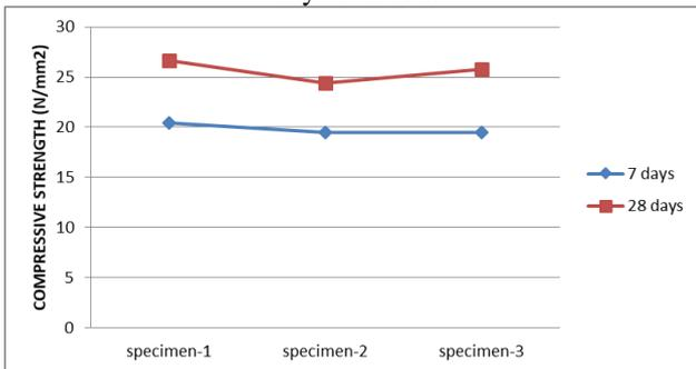
Fig. 3: Compressive Strength of M25 Concrete without Any Additions
