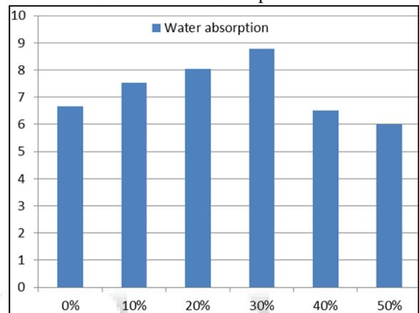
Fig. 5: Water Absorption Test
