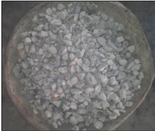
Fig. 1: Recycled Coarse Aggregate
