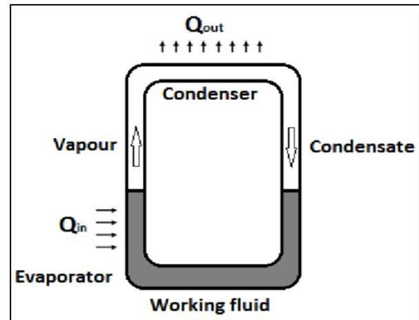
Fig. 1.1: two phase closed loop thermosyphon
