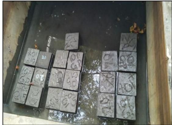
Fig. 7: Curing of Specimen
