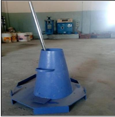
Fig. 6: Slump Cone Apparatus
