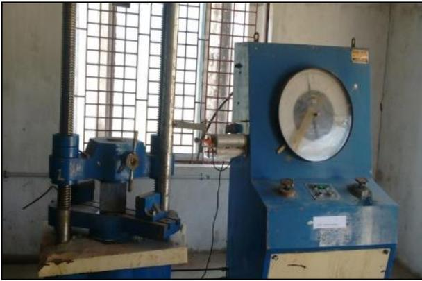
Fig. 8: Universal Testing Machine
