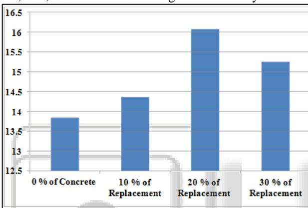
Fig. 9: Compressive Strength Test result after 7 days
