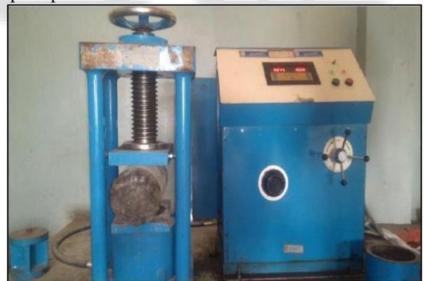
Fig. 12: Split Tensile Strength Testing Machine
