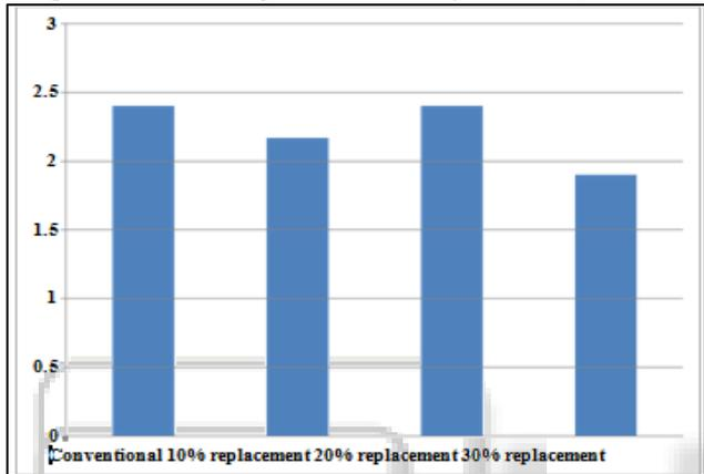
Fig. 15: Split Tensile Strength Test result after 14 days
