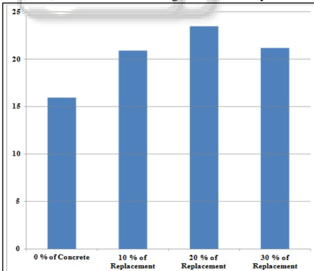
Fig. 10: Compressive Strength Test result after 14 days curing
