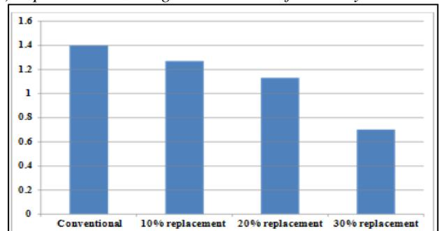
Fig. 13: Split Tensile Strength Test result after 7 days
