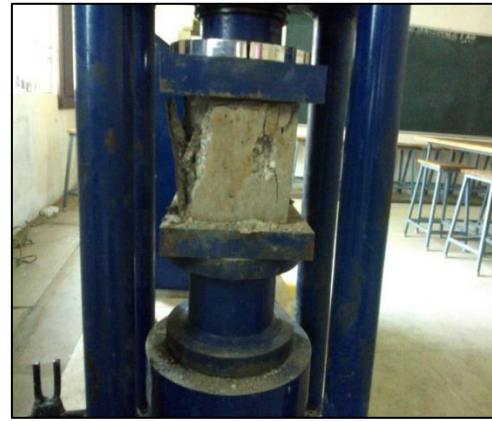
Fig. 3.2: Testing of cubes for compressive strength
