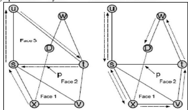
Fig. 6: Left, Packet Will Loop Around Face 3
