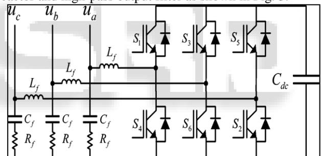
Fig. 3: Schematic Structure of a VSC
