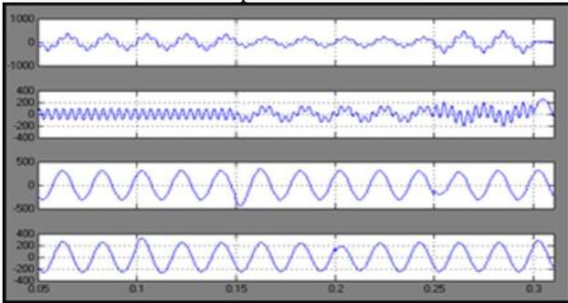
Fig. 12: Simulation Results for an Upstream Fault on Feeder2: BUS<sub>2</sub> Voltage, Compensating Voltage, and loads L<sub>1</sub> and L<sub>2</sub> Voltages.
