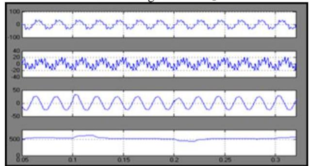
Fig. 11: Nonlinear load current, compensating current, Feeder<sub>1</sub> current, and capacitor voltage.
