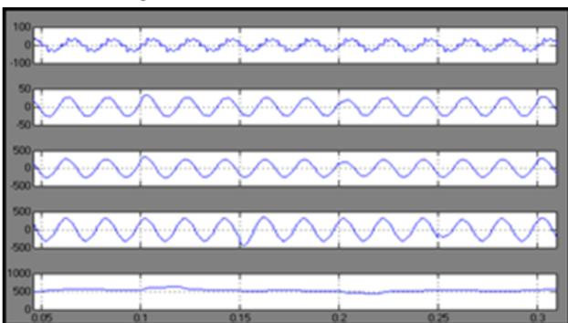
Fig. 13: Simulation results for load change: nonlinear load current, Feeder<sub>1</sub> current,
