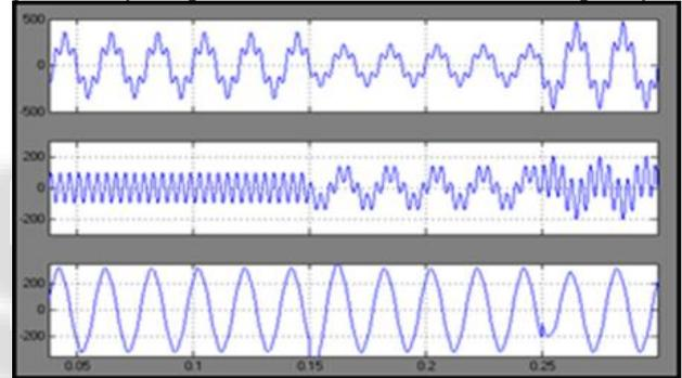
Fig. 10: BUS<sub>2</sub> voltage, series compensating voltage, and load voltage in Feeder<sub>2</sub>
