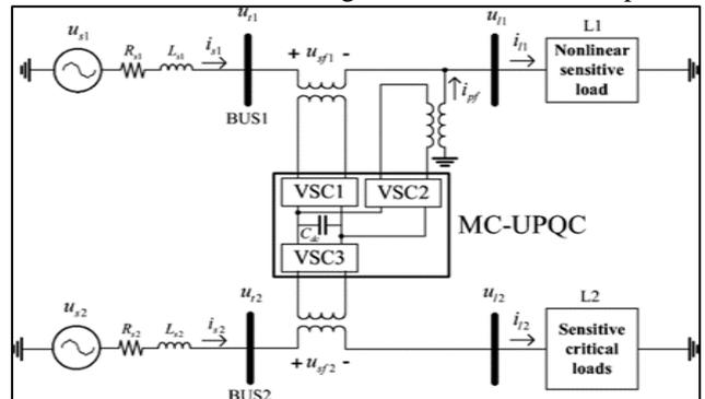
Fig. 2: Typical MC-UPQC used in a Distribution System
