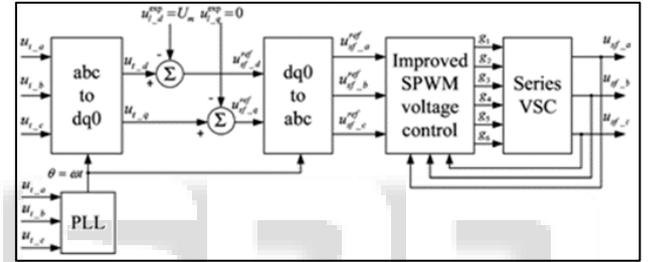
Fig. 5: Control block diagram of the series VSC
