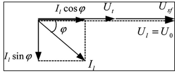
Fig. 7: Phasor Diagram of in phase Compensation (Supply Voltage Sag)
