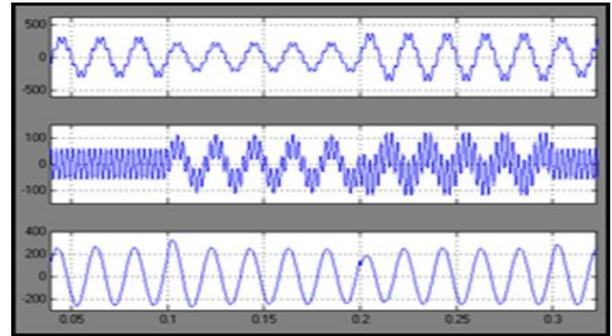
Fig. 9: BUS<sub>1</sub> Voltage, Series Compensating Voltage, and load Voltage in Feeder<sub>1</sub>.
