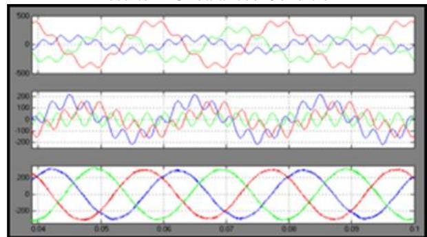
Fig. 15: BUS<sub>1</sub> Voltage, Series Compensating Voltage & Load Voltage in Feeder<sub>1</sub> under Unbalanced Source Voltage
