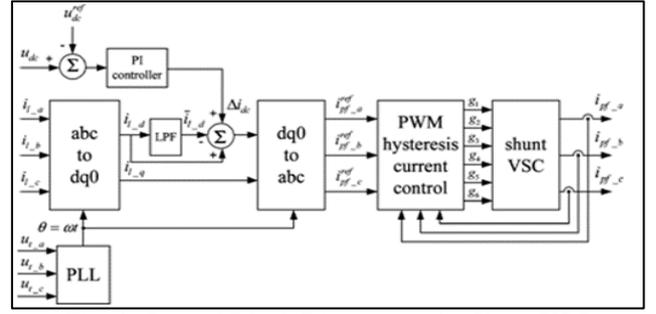
Fig. 4: Control Block Diagram of the Shunt VSC
