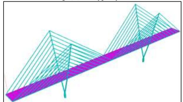
Fig. (C): Y-Type Pylon
