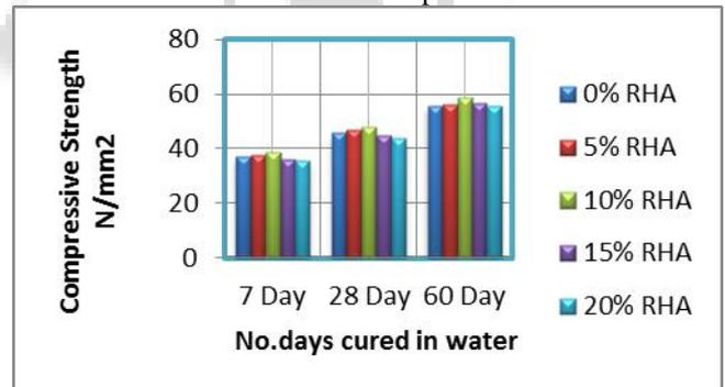
Graph 5.1: Compressive strength results cured in normal water
