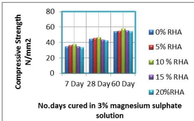
Graph 5.3: Compressive strength results cured in 3% magnesium sulphate solution
