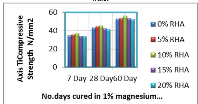
Graph 5.2: Compressive strength results cured in 1% magnesium sulphate solution
