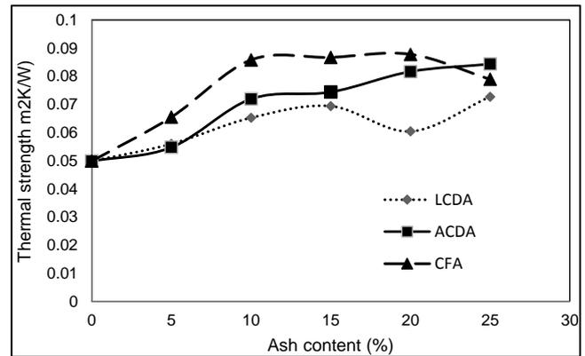
Fig. 10: Mortars thermal strength
