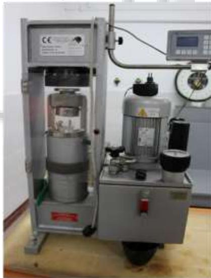
Fig. 6: Experimental device of compressive strength measurement
