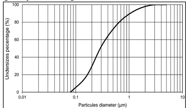
Fig. 3: Grain size curve of used sand
