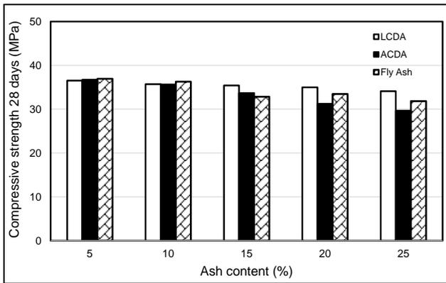
Fig. 7: Mortars compressive strength at 28 days
