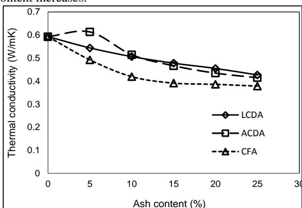
Fig. 9: Mortars thermal conductivity
