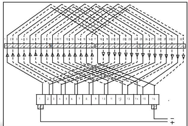
Fig. 4.1: Double Layer Lap Winding Diagram of PMG
