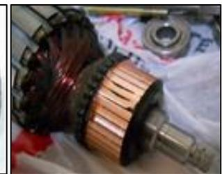
Fig. 5.2: PMG Armature
