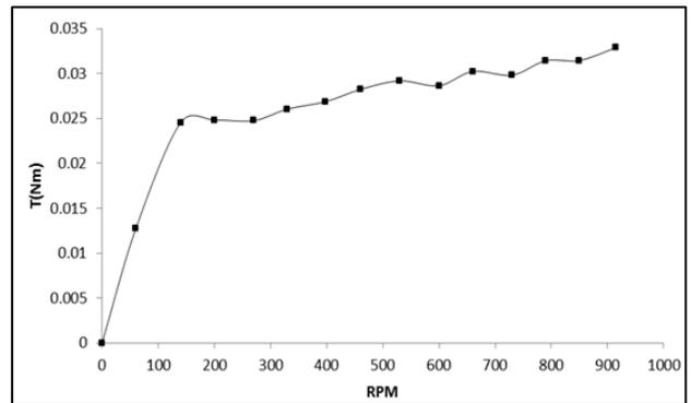
Fig. 6.5: Variation of Torque with Rotational Speed
