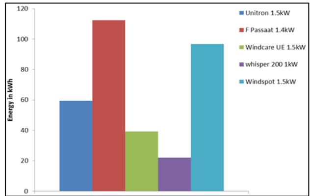
Fig. 6.4: Annual Energy Production by Different Wind Turbines
