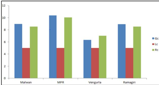
Fig. 6.1: Variation of Scale Parameter for Different Site by Different Methods
