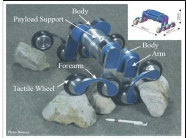
Fig. 2: All the parts touching ground
