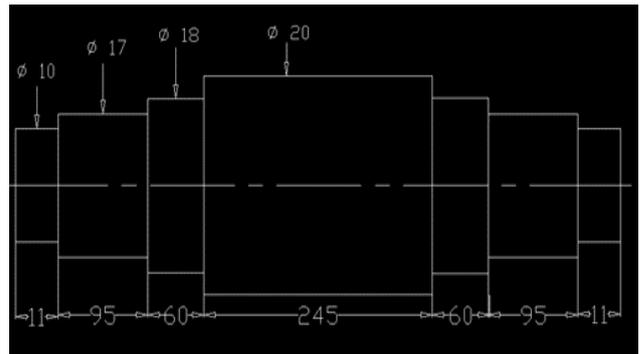
Fig 8: Driving Shaft
