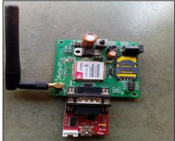
Fig. 7: GSM Modem
