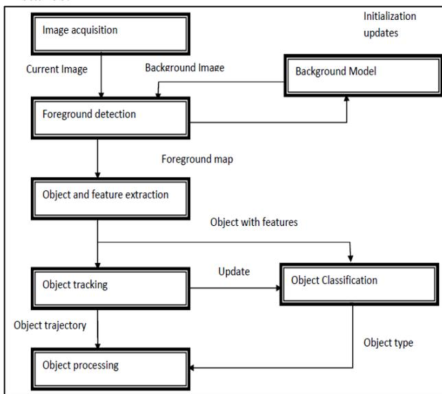
Figure 1 Video analysis block diagram
