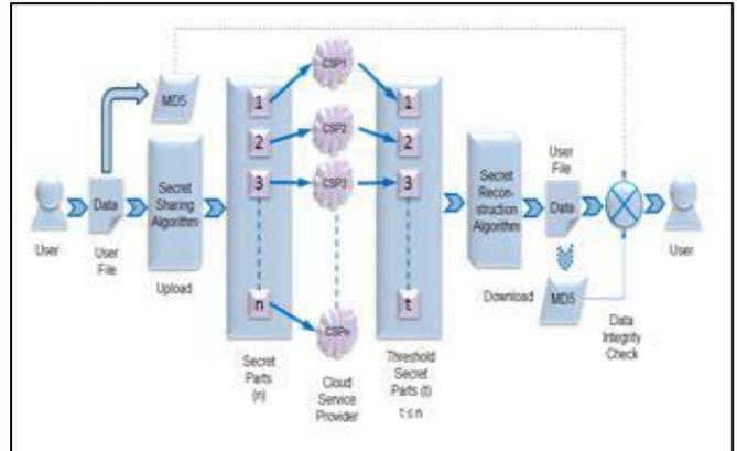
Fig. 3: Process of Secure Data Storage & Retrieval using Secret Sharing in Multi-cloud
