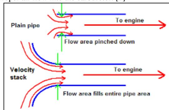
Fig. 1: Flow through pipe
