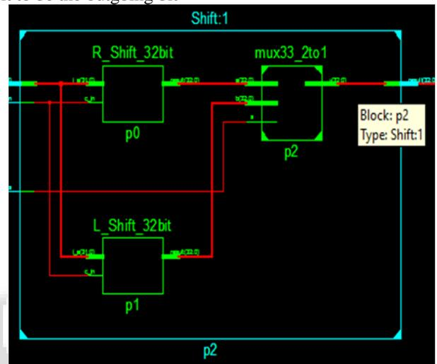
Fig. 4: RTL View of 32 Bit Shifter Unit
