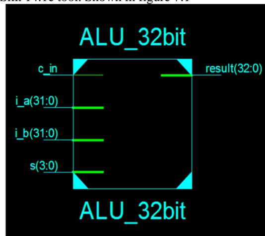
Fig. 1: RTL View of 32 Bit ALU
