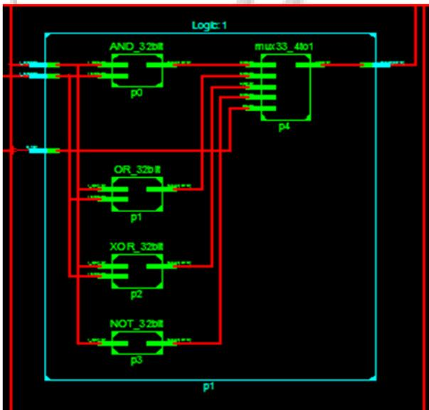
Fig. 3: RTL View of 32 Bit ALU
