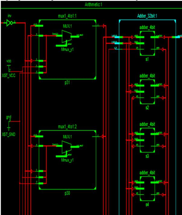
Fig. 2: RTL View of 32 Bit Arithmetic Unit
