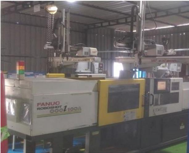
Fig. 1: Electronic 100ton Fanuc roboshot injection moulding machine
