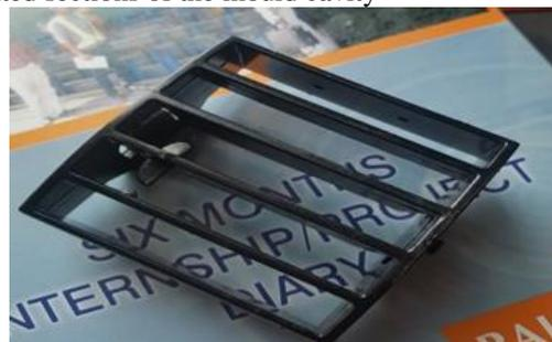
Fig. 3: Grill 609 (assemble parts of air vent housing)
