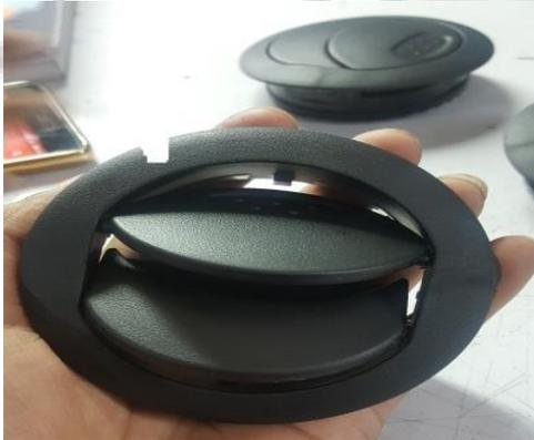
Fig. 5: air vent assemble part
