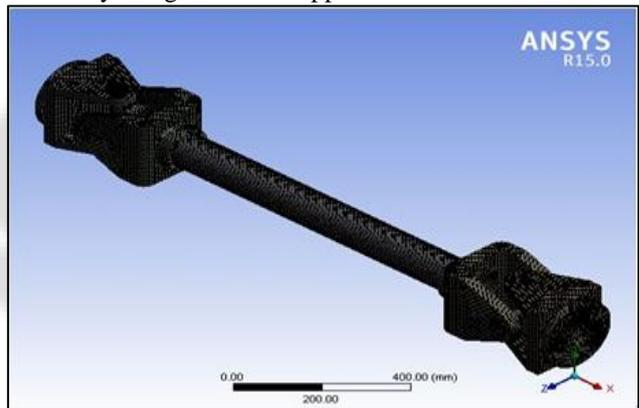
Fig. 2: Meshing of Cad Model using ANSYS
