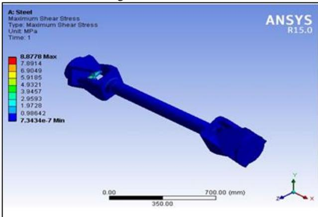
Fig. 5: Maximum Shear Stress
