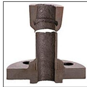
Fig. 9: High-Temperature Corrosion
