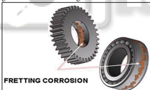
Fig. 8: Fretting corrosion
