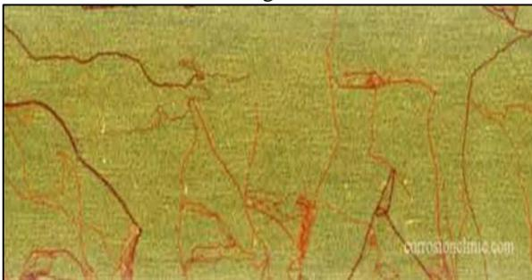
Fig. 5: Filiform corrosion of a tin-coated steel
