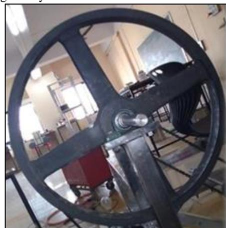
Fig. 3: Diameter of the flywheel is 61 cm
