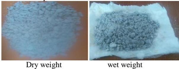
Fig. 11: Absorption test by incorporating diaper in the solution, the solution added on diaper and weight difference
