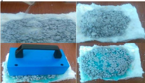
a) 40ml of water b) copper salt added c) 5kg of weight added d) check the color
