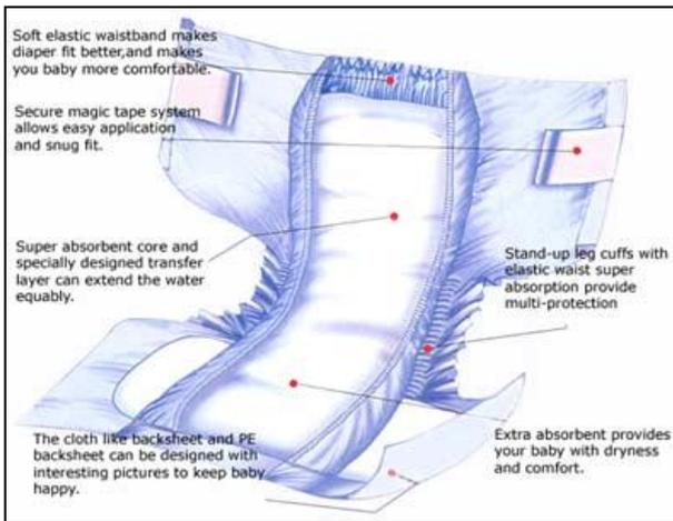
Fig. 1: Components of a disposable baby diaper.
