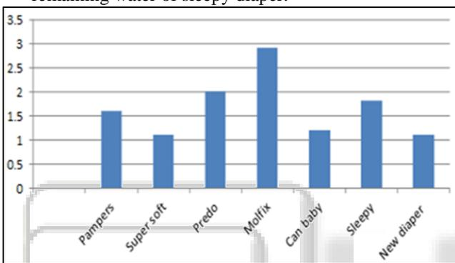
Fig. 8: Comparison of remaining water in ml in different diapers
