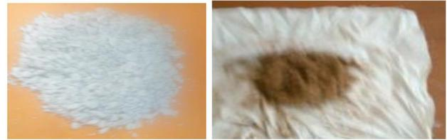
Fig. 6: Inside absorbent core
