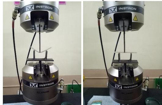
Fig. 3: Flexural test of composite material
