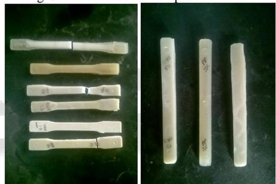
Fig. 4: Images of the specimens before and after loading (PP, ABS and HDPE).
