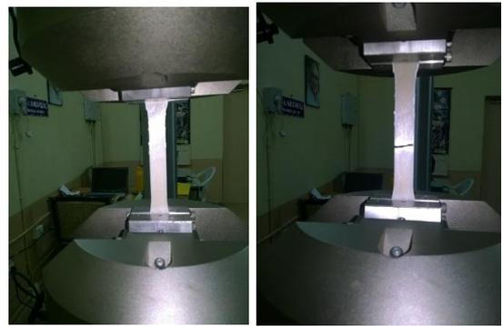
Fig. 2: Tensile Test of composite Material
