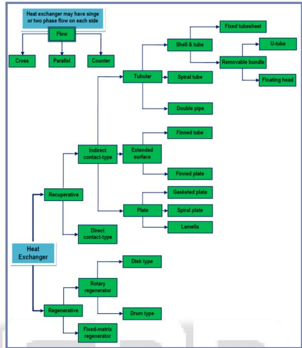
Fig. 1: Classification of heat exchanger
