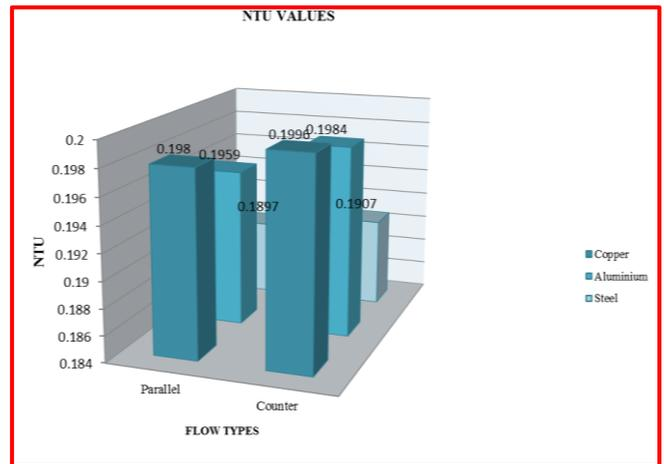
Fig. 8: NTU for different materials
