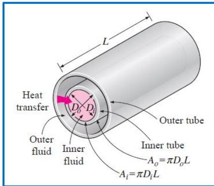
Fig. 2: Double pipe heat exchanger
