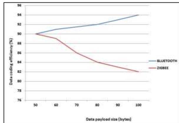
Fig. 9: Data coding efficiency comparison
