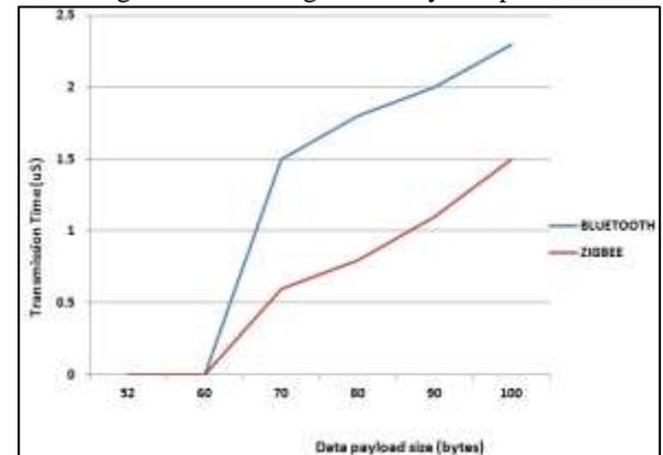
Fig. 10: Data transmission time of Bluetooth and ZigBee
