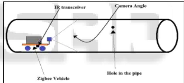
Fig. 6: Movement of vehicle through narrow pipe
