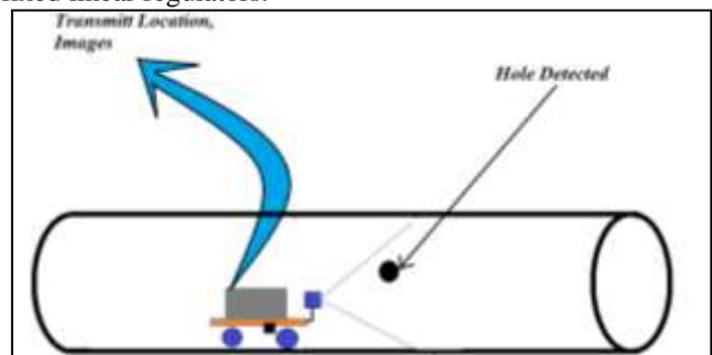
Fig. 7: Hole detection and data transmission
