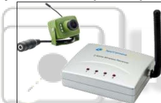
Fig. 4: Wireless camera and video transmitter
