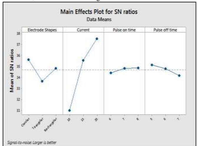
Fig. 7: Main Effects Plot for SN Ratio for MRR
