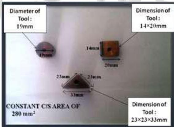
Fig. 2: Raw material pure copper (electrode shapes) as per required dimensions
