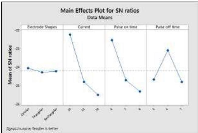
Fig. 12: Main Effects Plot for SN Ratio for SR
