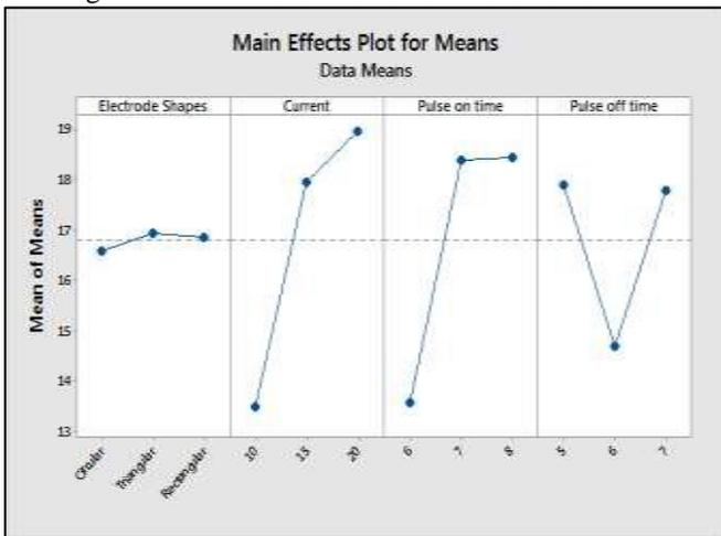
Fig. 13: Main Effects Plot for Means for SR
