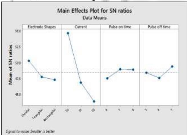
Fig. 9: Main Effects Plot for SN Ratio for EWR
