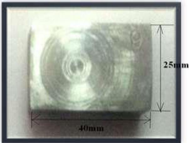
Fig. 1: Raw material SS 316 plates as per required dimensions
