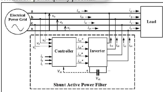
Fig. 1: Block diagram of Shunt Active Power Filter
