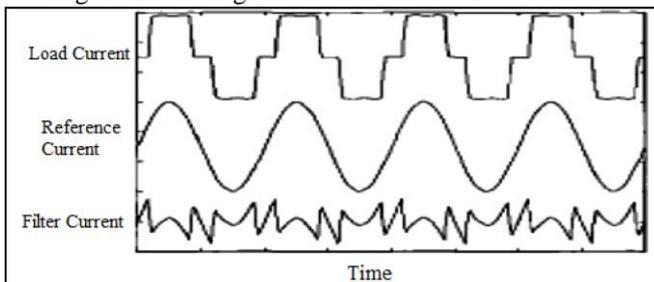
Fig. 2: Shunt active power filter-Shapes of load, source and desired filter current waveforms
